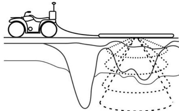
Fig. 3 – Schematic illustration of the ATV towing the Dualem-21s EMI-sensor. The dashed lines represent the 4 different signal response depths (i.e. 0-0.54 m, 0-1.03 m, 0-1.50 m and 0-3 m).
